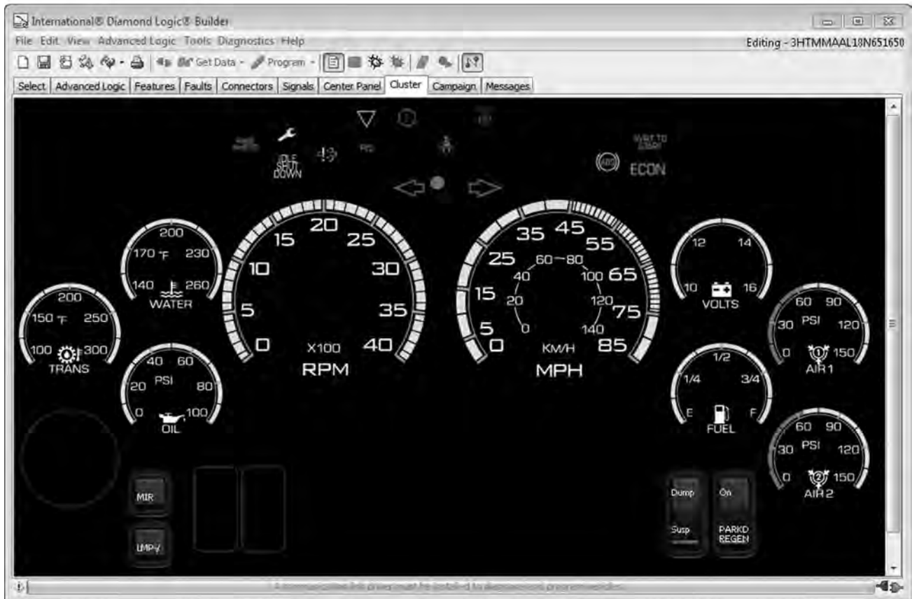
Figure 132 Cluster Tab with Two Vacant Switch Locations (Lower Left)
